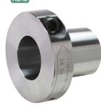
The shaft and the hub can be connected easily and quickly with 1 bolt. Since the concentricity is as accurate as 0.02 mm, this model is most suitable for applications that require high accuracy and where the device is frequently attached and detached. It is structured to be tightened from the radial direction to save work space.
